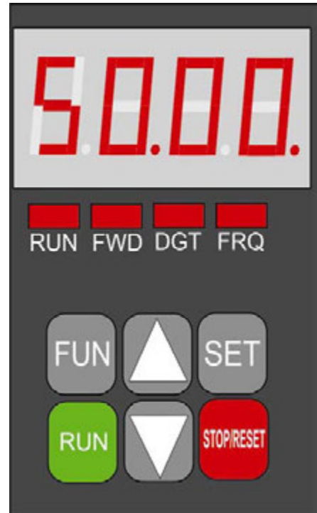
7-segment display, status LED and keypads
